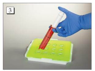
**Step 3.** Using a syringe pre-filled with ointment, fill each blister to about 65% capacity. We recommend placing the tip of the syringe against the bottom of the blister then slowly making a swirl pattern while moving the syringe upwards. This helps evenly dispense ointment and prevent splatter.
