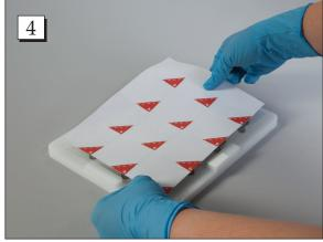
**Step 4.** First, remove the overlay from the blisters. Then peel the backing from the sheet of labels and match the notch markers on the labels with those on the blisters. Align the edges of the sheet with the edges of the blister tray and apply.
