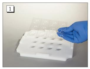
**Step 1.** To begin, remove a single blister tray from the stack and place it on top of the filling tray. If there are any detached blisters, place them in the missing areas on the fill tray.
